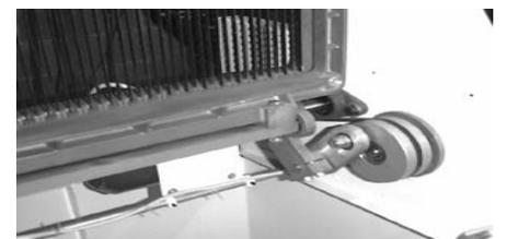
**KNIVES** they are at double frame with axial alternating movement
